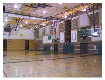
Motorized overhead mounted backstops from <u>Performance Sports Systems</u> included glass backboards and breakaway rims.
