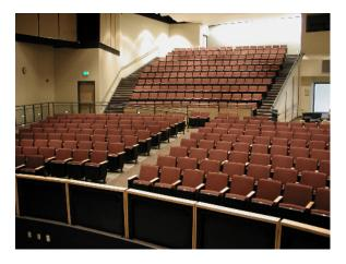
Telescopic bleachers from Interkal feature aisles transitioning from main floor to balcony and fully automatic self storing aisle rails.
